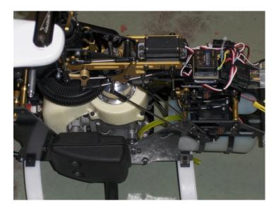
Figure 1. Power plant used on mini-UAV helicopter
