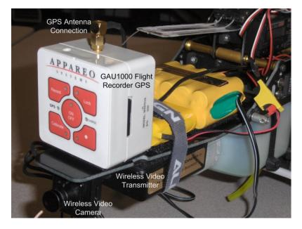
Figure 2. Mini-UAV payload (flight recorder, wireless video camera/transmitter, battery pack)
