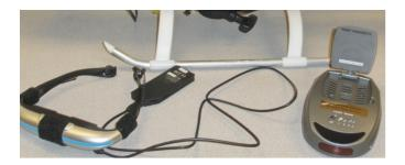
Figure 4. Ground station receiver and headset
