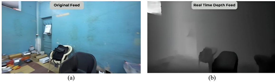
Figure 7. QUADRESCUE perception system output (a) original RGB feed from Intel D435i camera and (b) real-time depth feed visualization
