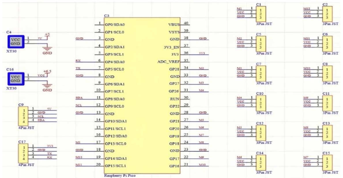
Figure 2. Circuit schematic of QUADRESCUE’s servo control system based on Raspberry Pi Pico microcontroller
