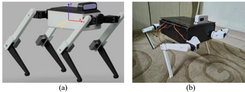
Figure 6. QUADRESCUE robot design implementation (a) 3D model of complete assembly with coordinate system (b) actual working prototype
