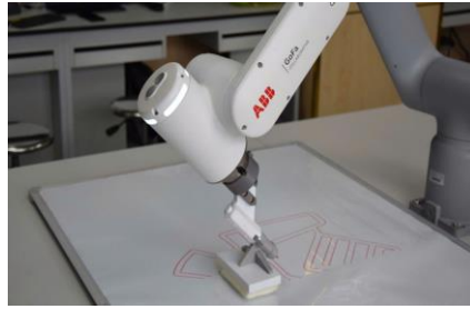
Figure 9. Configuration of the GoFa robot with the integrated cleaning pad mounted at the end-effector
