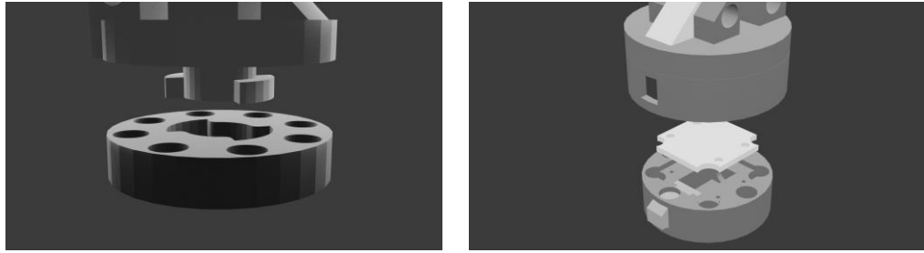
Figure 2. The socket flange with a spring-loaded locking mechanism for quick, screw-free tool attachment to the robot's end-effector
