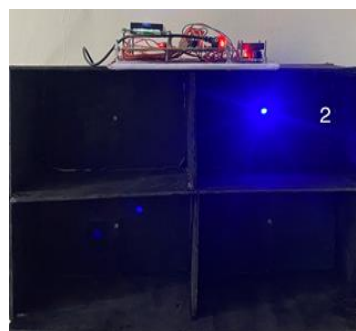
Figure 5. LED above Shelf 2 glowing for selected book "Elon Musk," demonstrating pick-to-light guidance
