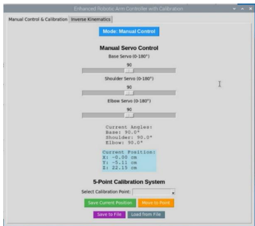
Figure 5. RA control calibration and inverse kinematics
