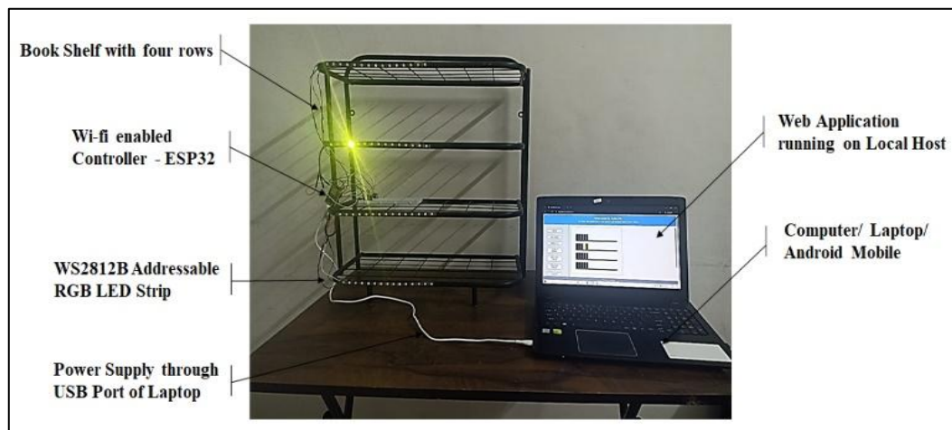
Figure 1. Developed IoT enabled LED addressing technique
