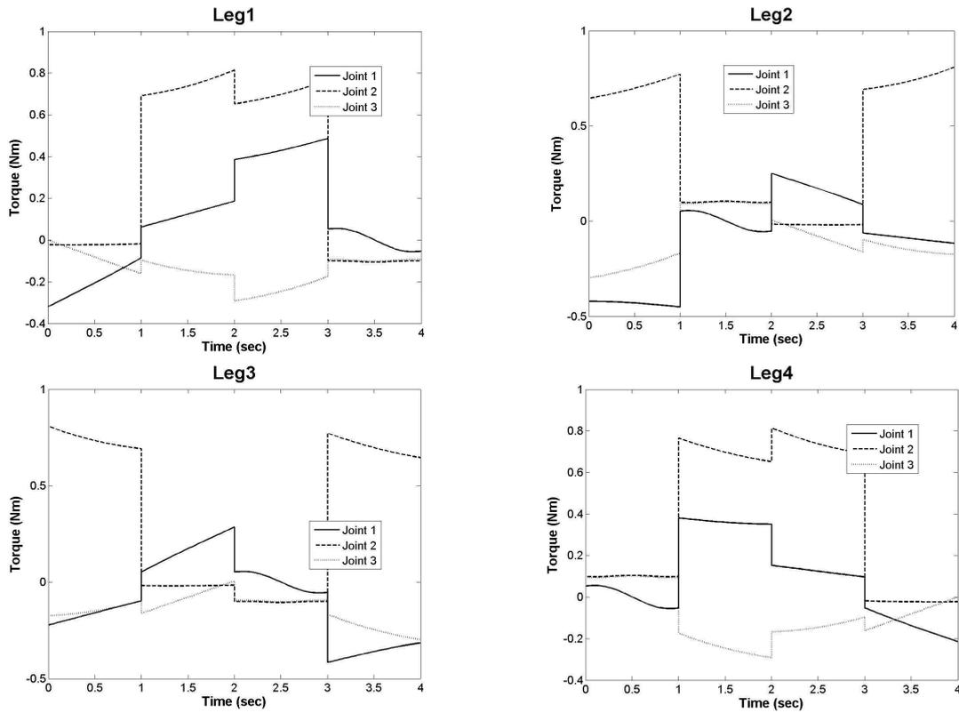
Figure 9. Variations of joint torques at each joint of the legs obtained by Approach 2
