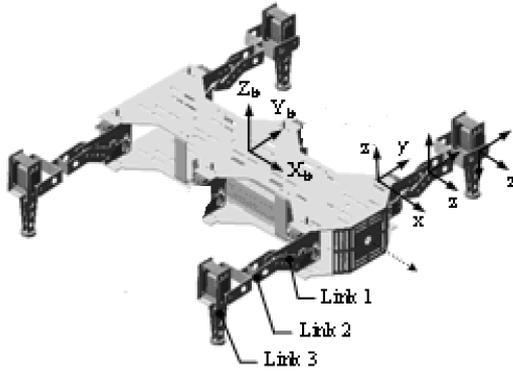
Figure 1. The model of four-legged robot
