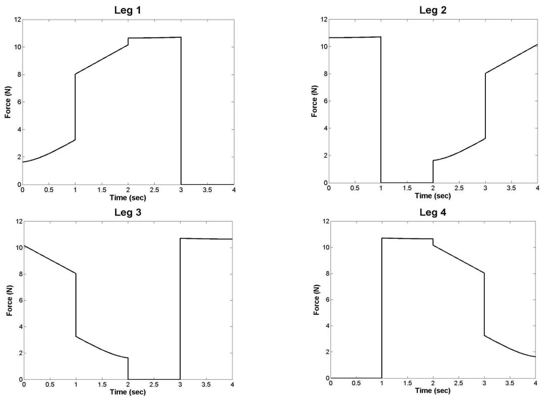
Figure 6. Distributions of feet forces obtained by approach 2
