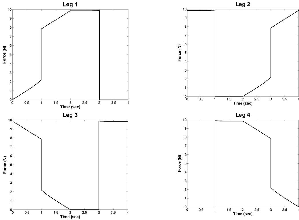
Figure 7. Distributions of feet forces obtained by approach 3
