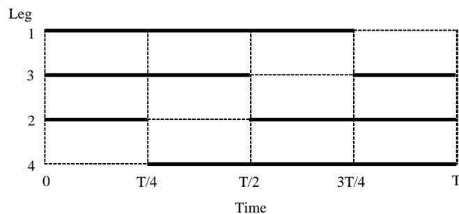
Figure 3. Gait diagram with duty factor 3/4
