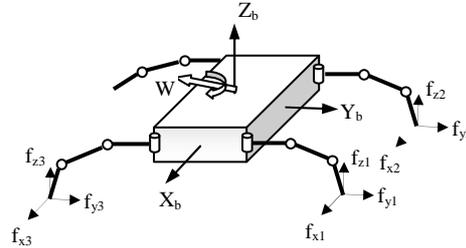
Figure 4. A schematic view showing feet contact forces acting on the robot
