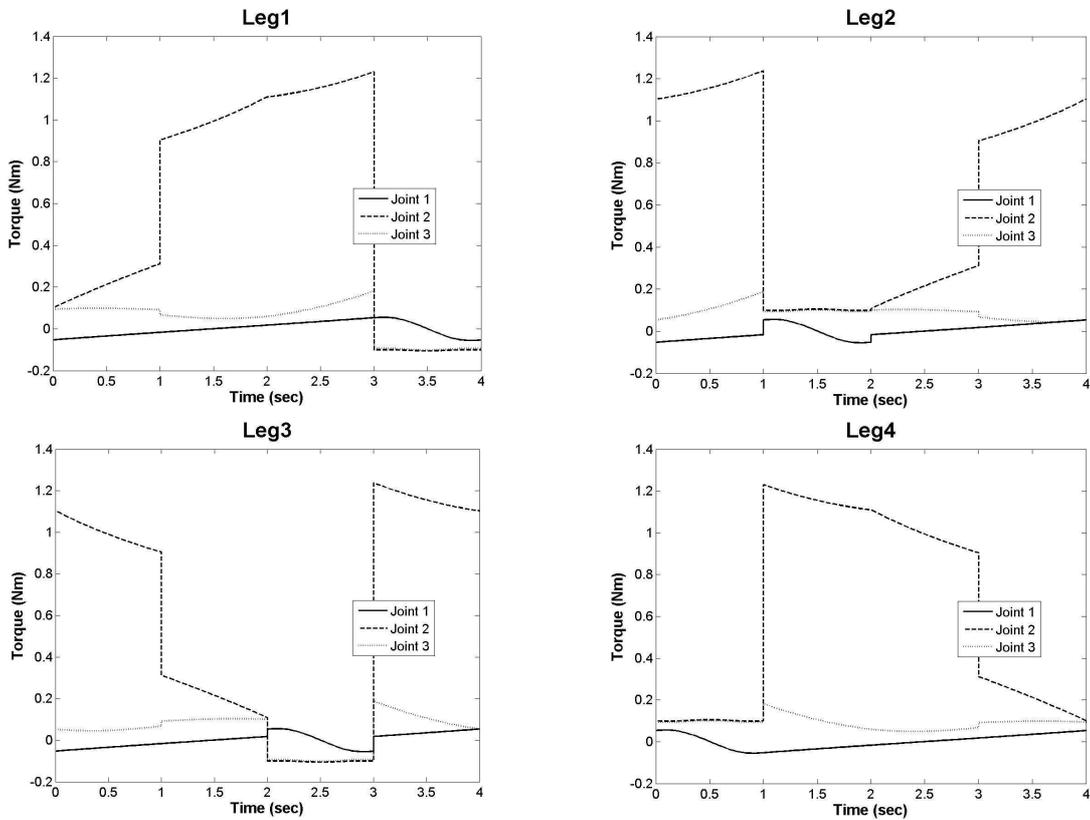
Figure 8. Variations of joint torques at each joint of the legs obtained by Approach 1
