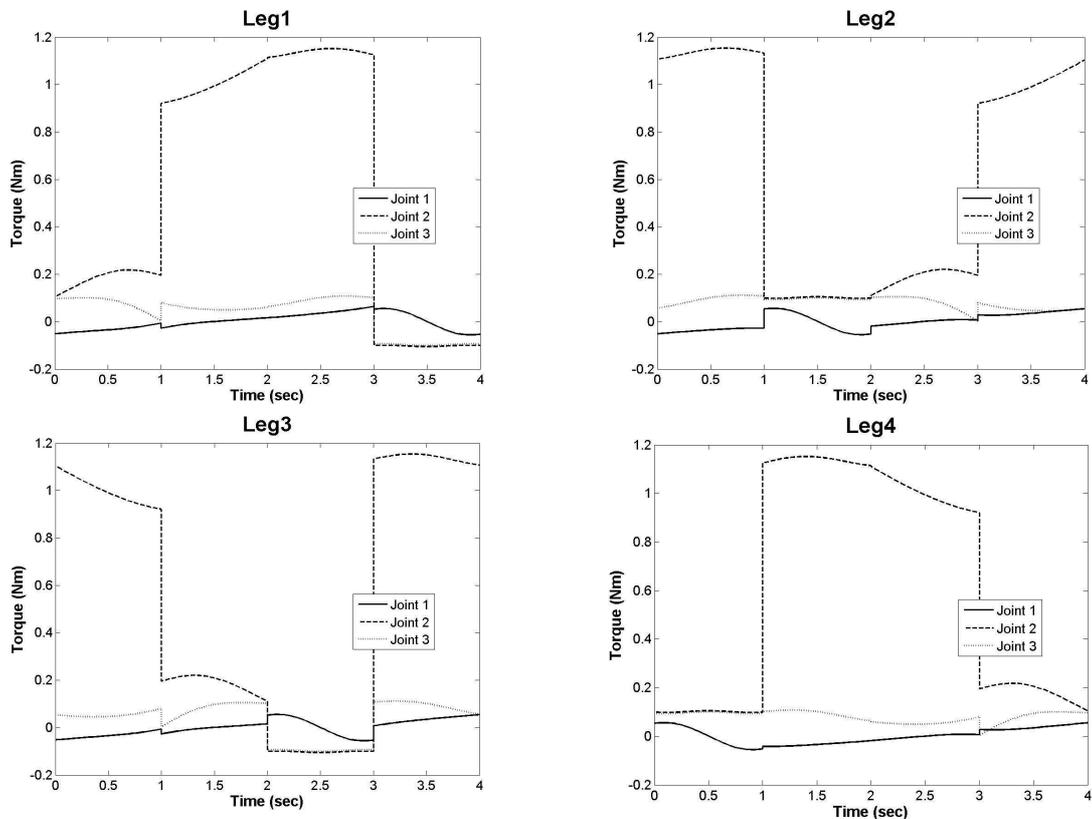
Figure 10. Variations of joint torques at each joint of the legs obtained by Approach 3
