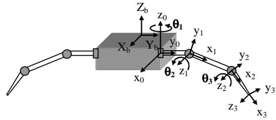
Figure 2. D-H representation of link frame
