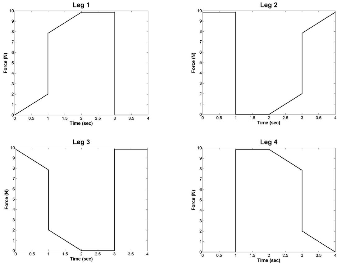
Figure 5. Distributions of feet forces obtained by approach 1
