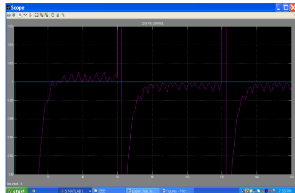
Figure 16. system responses with feed forward type 2DOF controller with Zoom
